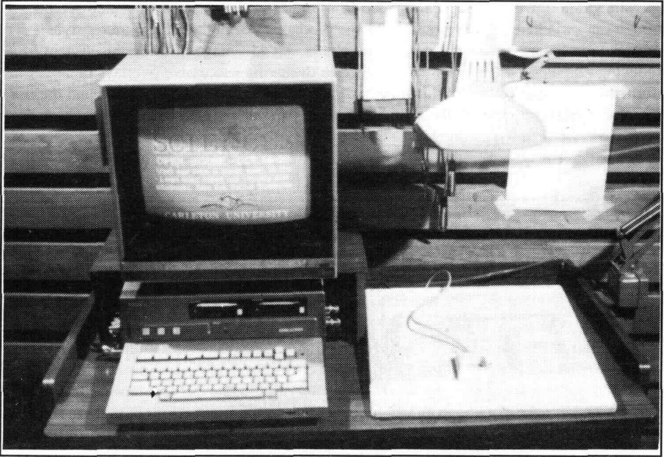
Figure 1. Graphics Creation Workstation Consisting of Sony Microcomputer, RGB Monitor and Graphics Tablet.
