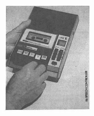
A high-quality, sturdy audio cassette unit with a speed range that may be varied by the user from 60 percent of normal speed to 2 1/2 times normal speed without pitch distortion.
