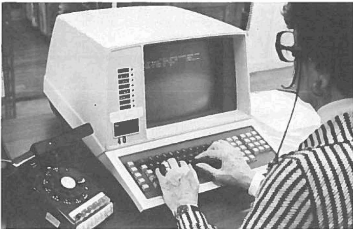
All bookings are received by phone and typed into the VUCOM II terminal. A dedicated phone line connects the terminal to an IBM computer three kilometres away.
