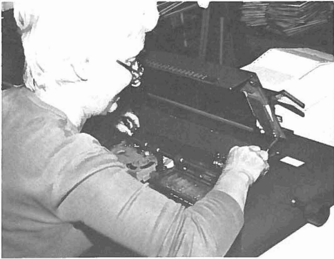
Changing platens in the typewriter.
