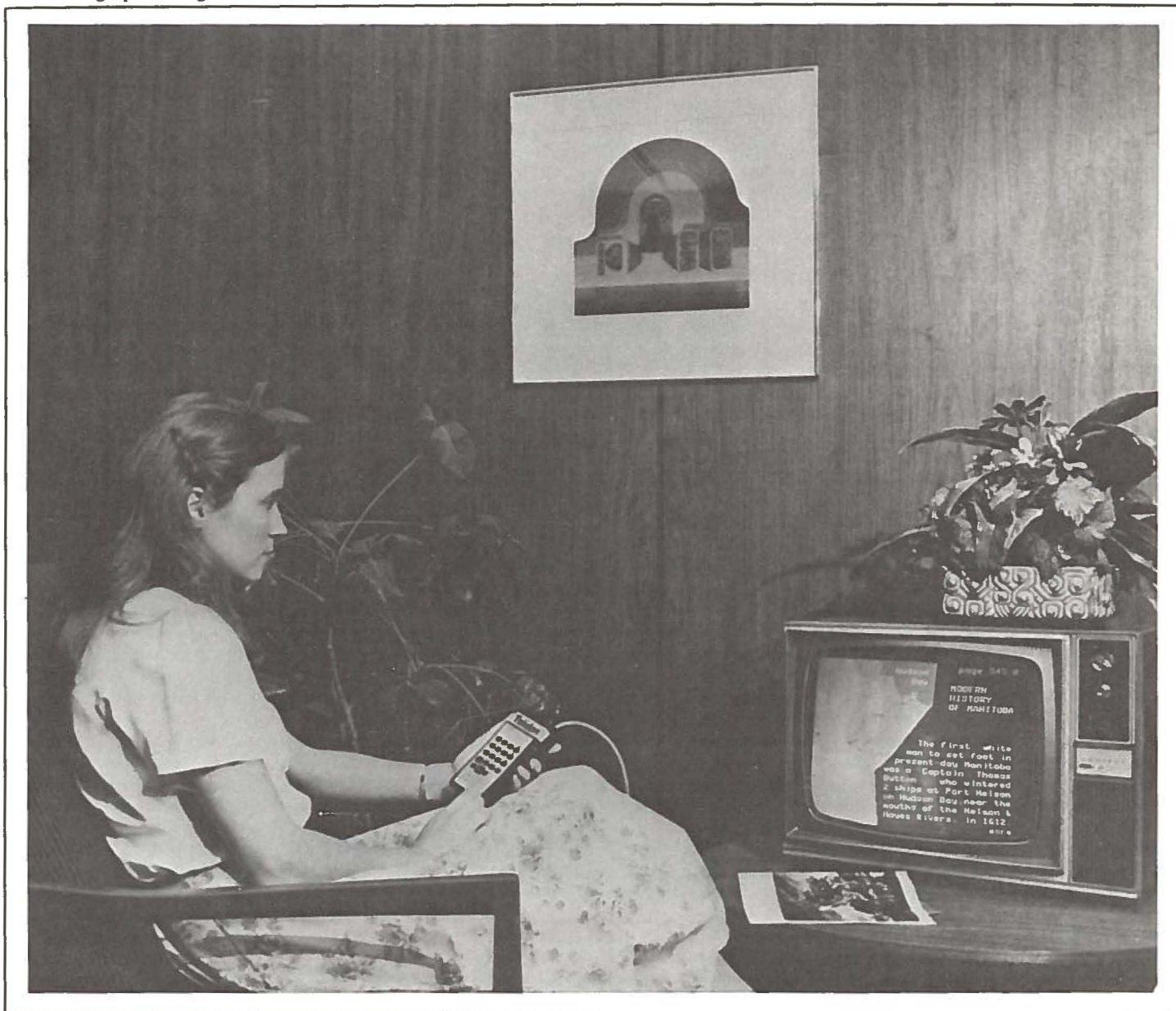
Figure 2. Telidon pages of information can presently be accessed by a hand-held key pad. Information pages can combine both text and graphic images.
